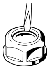
Figure 5-7 Stripping a seal ring
