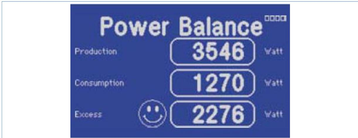
A "smiley" emoticon "☺" is shown in the display when power is being directed into the mains supply for remuneration
