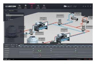
Space Explorer provides easy-to-use browsing and quick control with the convenient inter-floor movement and shows transition without moving into other menus
