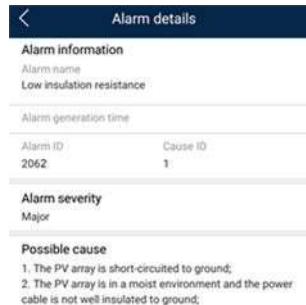
Figure E-1 Alarm details
